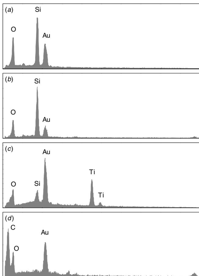
**Figure 4.** EDS composition analysis. (a) and (b) Spectra for SiO<sub>2</sub> SD structures obtained by pyrolysis and acid-etching, respectively. (c) Spectrum for TiO<sub>2</sub> SD structures. (d) Spectrum for scales.
