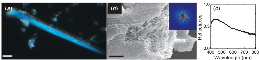
**Figure 3.** Optical and structural characterizations of the fabricated TiO<sub>2</sub> SD structures. (a) Optical microscopic dark-field image. (b) SEM image. The inset is the spectrum of two-dimensional Fourier transform analysis. (c) Measured reflectance spectrum. Scale bars: (a) 10 μm and (b) 2 μm.
